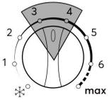
Most combi boilers don't have the temperature displayed around the radiator temperature dial. You'll want to adjust the target radiator temperature to about **60°C**.
